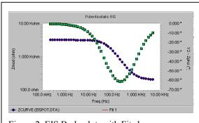
Figure 2. EIS Bode plot, with Fit shown.
