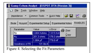
The graphical description of the circuit model used to fit the data can be copied
